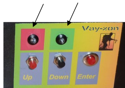
Central Recharge Unit front panel showing team base connected lights
